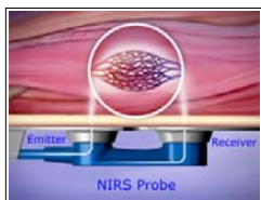
Figure 1 – NIRS Probe measures changes in light reflected from blood and other tissues.
